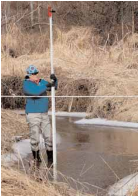
THI's Lisa Marr measures the depth of an eroded stream in Virginia to help formulate a sustainable restoration design.
